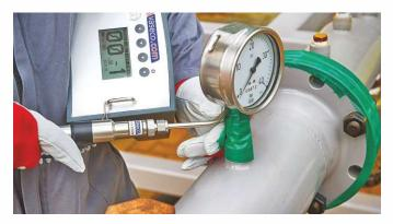
leak detection method used to identify even small leaks in pipelines or other systems.
